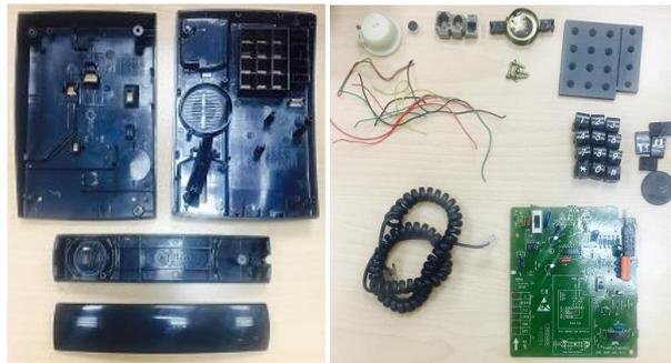
**Fig. 5** Dismantled Wireline Telephone Parts Consisting Of Plastic Casing And Components, Wires, Magnet, Electrical Components (Switches, Capacitors, SMD Components), Metal Parts (Screws, Plates) And Printed Circuit Board.
